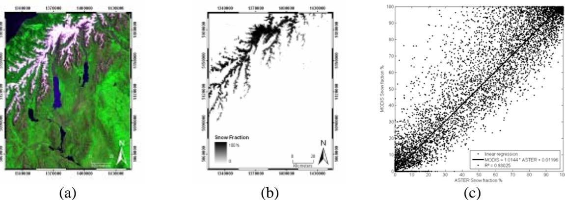
**Figure 1** - Estimation of the Snow fraction for granule 2002365.2235 (Upper Waitaki Area, South Island of New Zealand, 31 December 2002 22:35 GMT): (a) False color RGB composite from bands 1,2 (250m) and 3 (fused to 250m). (b) Result of unmixing using bands dataset at 250m. (c) Snow fraction from MODIS 250m fused bands versus reference.
